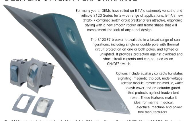
The 3120 series includes models rated from 0.1 to 20A with voltage ratings of 240V AC and 50V DC. Single-pole versions for up to 30A are also available by special order. Operating temperature range is -22 to +144°F (-30 to +60°C). All models are fully approved by UL, CSA and VDE.
