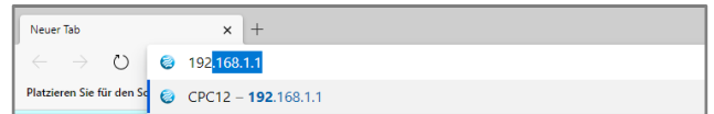
Image 6: Typing the default IP address of the CPC12 webserver in the search field
