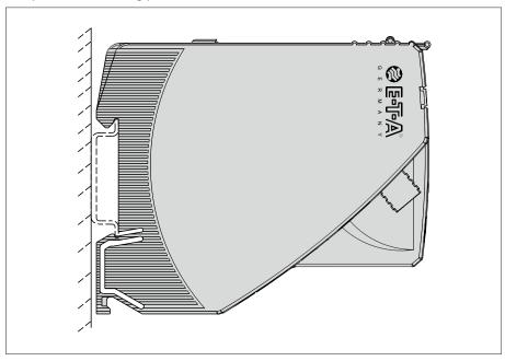
Figure 6: Mounting position of the EM12D-TIO
