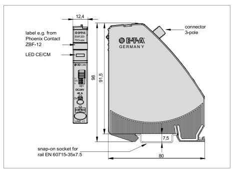
Figure 2: Dimensions of the EM12D-TIO
