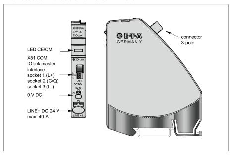
Figure 3: EM12D-TIO status indication and terminals
