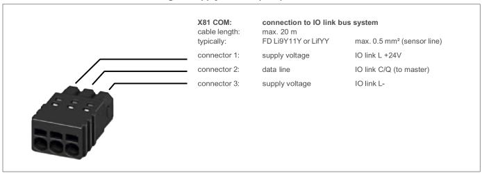
Figure 8: IO link connector
