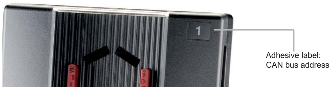
Figure 9: Labelling the CAN bus address on the module
